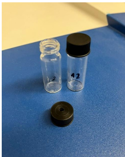
Figure 12: A representation of the glass vials used for PhotoCube measurements with and without a hole on the top of the vial.
